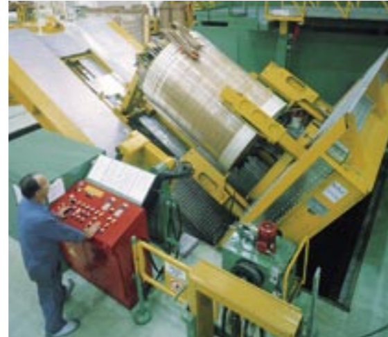
An automated tilting cradle is used to raise the windings from the horizontal to the vertical position in order to ensure that the larger windings retain their perfectly round shape when the metal mandrel is removed.
